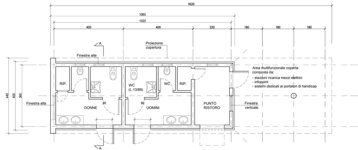
PROGETTO: PIANTA LIVELLO PISTA CICLABILE - SCALA 1:500
